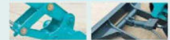
Bucket: Cast-iron idler link provide greater strength. Dozer: Box construction dozer supports provide greater strength.
