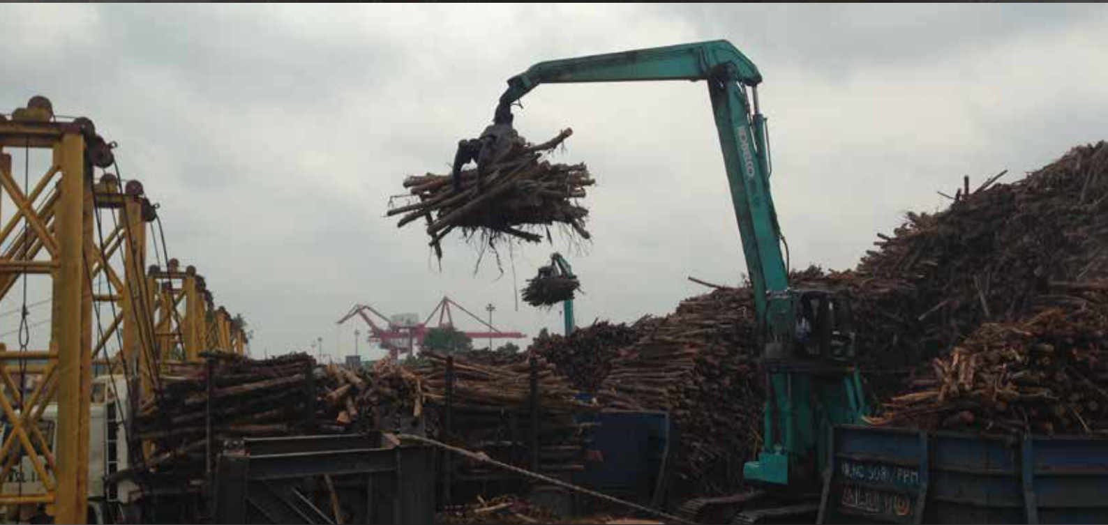
Randalls 2.0m2 Grapples working on Barge unloading Indonesia
