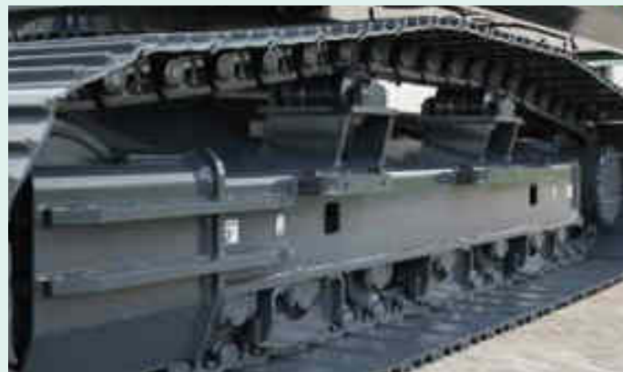
Track guides installed in three places
