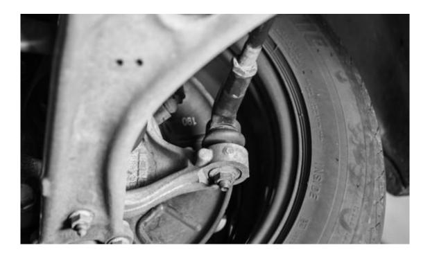
LEMFÖRDER tie rods for passenger cars, vans and light commercial vehicles ensure precise steering and safe handling. The forces introduced into the steering gear are transmitted via the inner axial joint through the tie rod to the outer ball joint, the tie rod end piece. A thread in the middle of the wheel allows for sensitive adjustment of both wheels.
